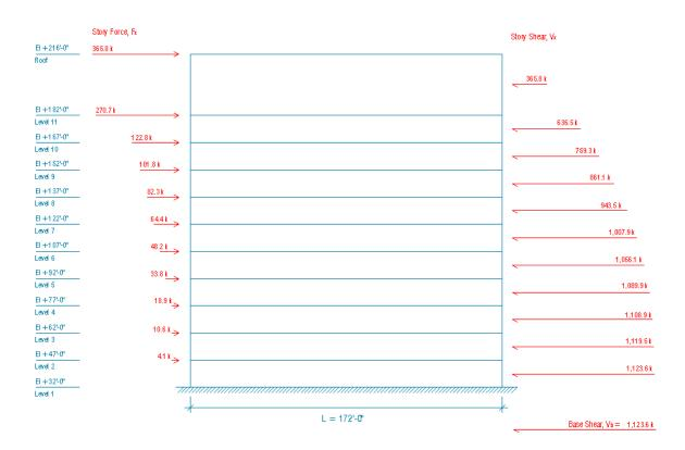
Wind Pressures on North-South Frame  $B = 172 \ \text{ft}, \ L = 200 \ \text{ft}$
