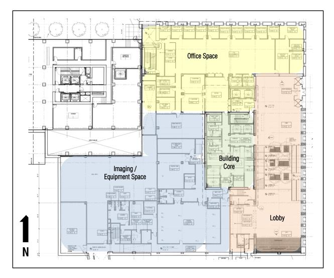
Figure 5: Level 1, Architectural Plan
